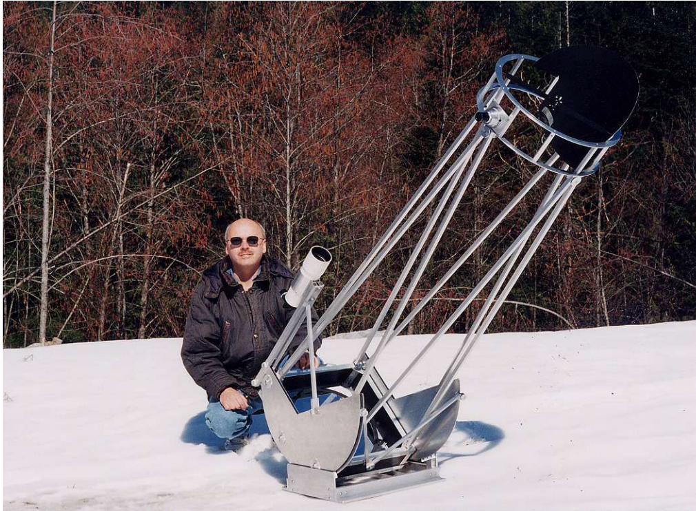
Figure 2 – Gary Wolanski's 16" 40 pounder, an almost-all aluminum Dobsonian.
