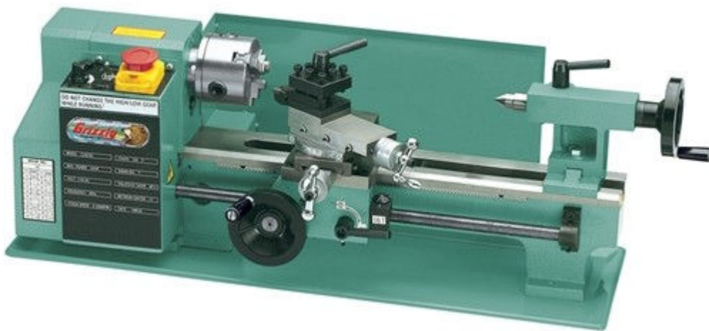
Figure 5 - One of the popular imported "7x12" mini-lathes. Courtesy Grizzly Tool.
