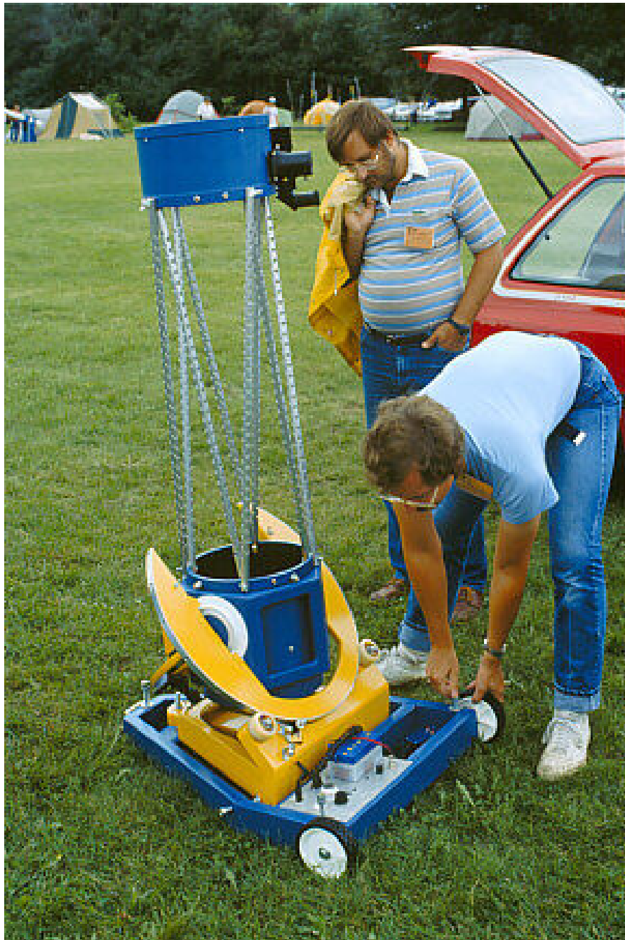
Figure 6 - A small split ring mount, lightened by drilling holes in the truss tubes.
