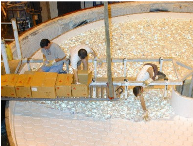
Figure 3 University of Arizona Mirror Lab workers load glass into a telescope mirror mold prior to melting and spin-casting.
